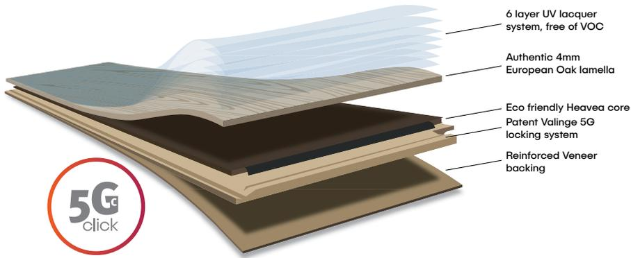
CLIC Oak's joining system allows for quick and easy installation and can be used for both floating and glue down applications. Installing CLIC Oak is simple. It's based on a single fold down action saving time and costs. The 5G locking technology is an essential component to CLIC Oak's design, guaranteeing superior locking strength and ensuring no separation forces during or after installation.
